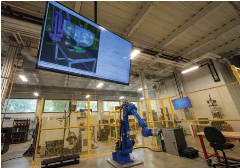
Pictured above: Early stages in the development of a robotic machining research cell. The monitor shows a virtual machining process in-the-loop with the physical robot. Pictured in the right top corner: A robotic sheet forming cell uses digital image correlation measurements in-the-loop to create high accuracy freeform sheet metal parts.
